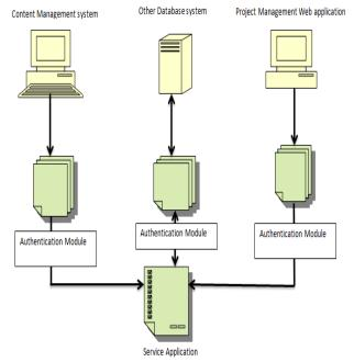
Fig 3.1: Interaction of service application to fetch data from "CMS" to "PWA"
